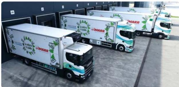
MARR has 9 liquid natural gas (LNG) vehicles, large-capacity trucks intended for long distances, used for the distribution sections from the logistics platforms to the distribution units.
